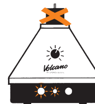
Caution! Causes burns! Never leave filling chamber on VOLCANO
